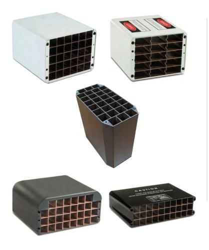
Kanfit manufactures chaff and flare magazines by RTM. This process improves magazine accuracy, extends durability and enhances reproducibility. There are zero failure points because there are no seams, bonding, assemblies, etc. Produced in one piece and in one-shot with the metallic inserts embedded into the component, Kanfit chaff & flare magazines are significantly lighter in weight than those made from metals.
